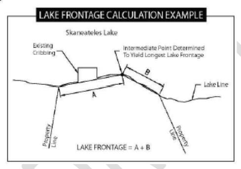
LAKE LINE/Mean High Water Mark— The shoreline of Skaneateles Lake when the lake level is 865.02 feet (National Geodetic Vertical Datum 1929), the legally established elevation to which the City of Syracuse may raise the level of the lake. (The corresponding level using City of Syracuse datum is 863.27 feet.)
